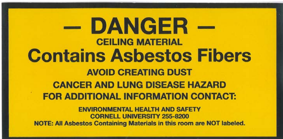
Label 4 – Asbestos containing ceiling material label (i.e. spray-on ceiling ) (Black lettering on yellow background)
