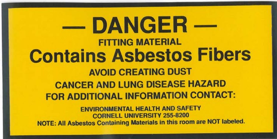
Label 3 – Asbestos containing fitting material label for utility systems. (Black lettering on yellow background)
