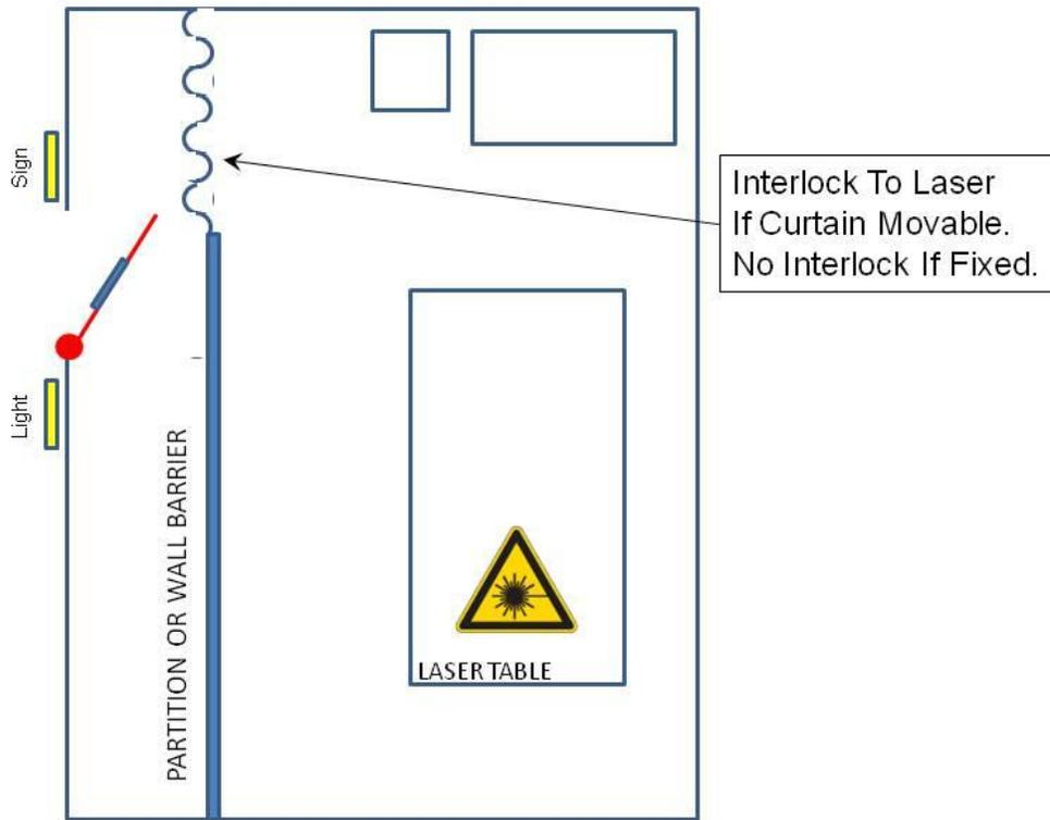
Figure 7 – Example of High Power Class 3b or Class 4 Entryway Protection
