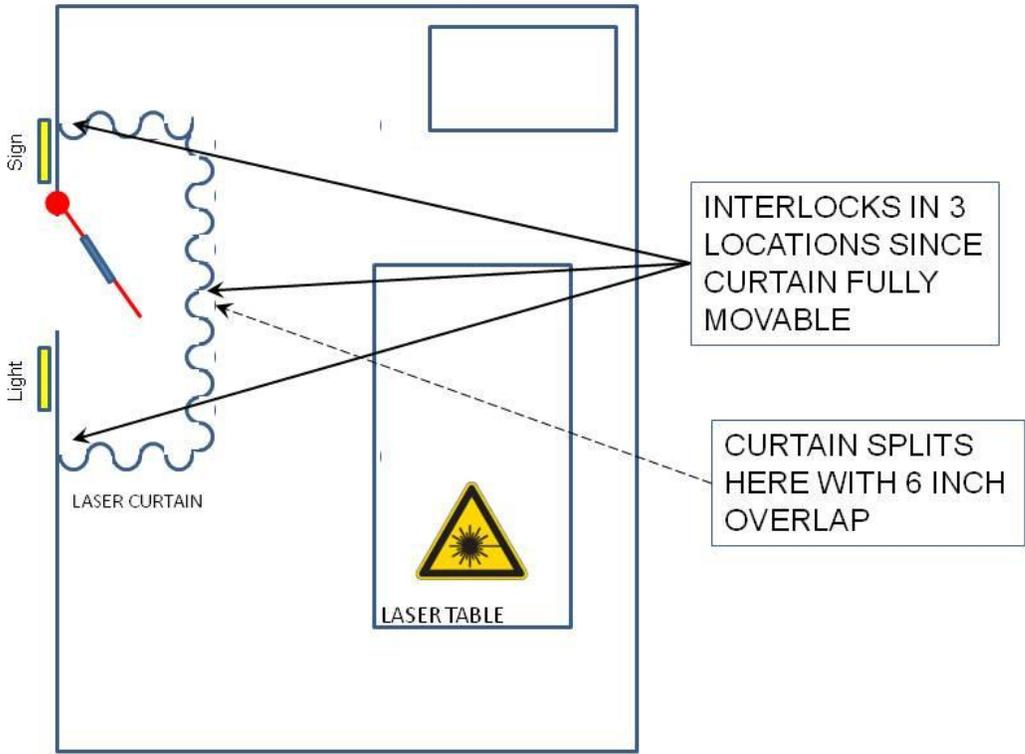
Figure 6 – Example of High Power Class 3b or Class 4 Entryway Protection
