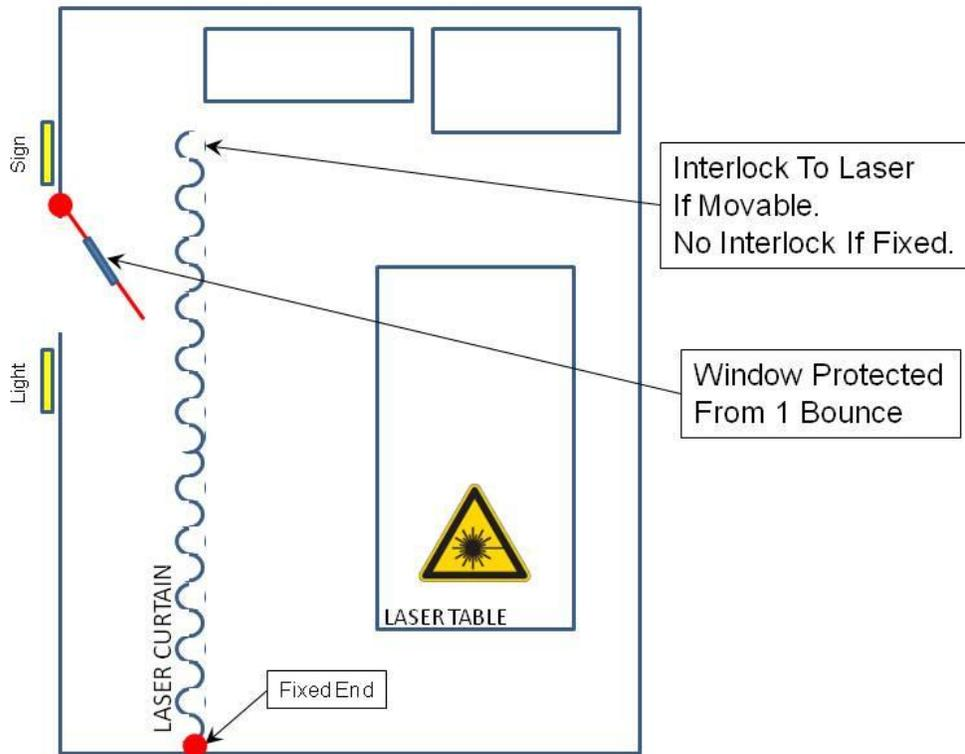
Figure 5 – Example of High Power Class 3b or Class 4 Entryway Protection
